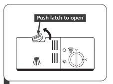
1 Press the release latch on the detergent dispenser to open the cover.
