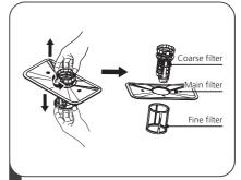
The fine filter can be pulled off the bottom of the filter assembly.
