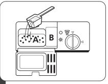
Add detergent into the larger cavity (A) for main wash. For more heavily soiled wash loads, also add some detergent into the smaller cavity (B) for release during pre-wash.
