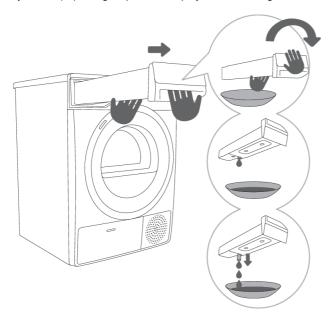
1 Pull out the condensate tank from the dryer (using both hands as shown in the figure), then turn it upside down over a washbasin, sink, or any suitable vessel.
