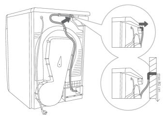
Release the hose from the holder on the back wall of the dryer (left hand side, below the top cover).
