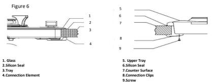
The range is equipped with a seal to prevent the liquids through the cavities into the cabinet. In order to place this seal, adhere the seal as shown in the figures above. Turn the range upside down and remove the protective tape of the rubber seal and adhere it to the range; both ends of the seal should meet each other. Install the mounting sheets as shown in figure 5 by help of screw. And place the range in the opening on the counter.
