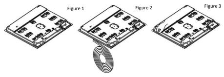
Turn upside down range in the Styrofoam in the package and apply the silicon.
