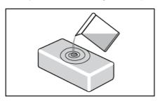
Fill the box with 16.9 fl oz (0.5 l) of tap water and place it in the relevant zone. There are no preferrable positions, as long as it is placed in the correct zone.
