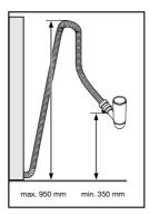
The drainage hose may be extended by a maximum of 3 m (the total length of the drainage hose must not exceed 4.5 m). Any joints and connecting pipes must have an internal diameter of at least 14 mm.
