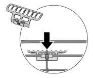
Fit the cutlery holder to achieve maximum loading capacity. (Found inside the enclosed plastic bag.)
