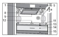
The serving area (zone B) is a temperature zone between the top (5) and bottom (15) insulation barrier. It allows you to bring the wine on ideal consumption temperature, and to prepare in advance everything you need for quick and top-notch wine serving: chilled wine glasses, space for already open bottles, decanter, and other accessories (bottle openers, wine pourers/spouts, stoppers ...).
