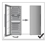
4. Adjust the door position until the edge of the door is parallel to the side of the housing.
