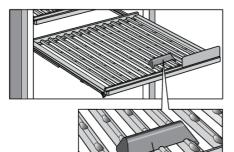
The wooden bottle shelf with moon shaped recesses allows you to load the bottles onto the shelf cross-wise.
