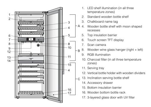
There are two insulation barriers inside the wine climate cabinet: top insulation barrier (5) and bottom insulation barrier (15). Thus, the inside of the wine climate cabinet is divided into three temperature zones: A, B (serving area) and C. This allows storage and immediate serving of different types of wine.
