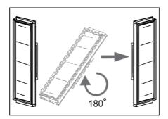
9. Carefully rotate the door by 180 degrees.
