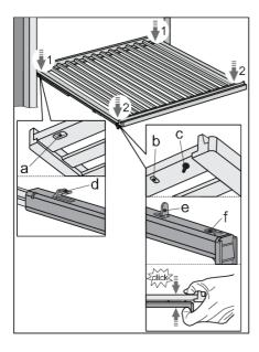
To replace a shelf onto the rails again, use the grooves (a, b) and pin (c) on the back and front side of the shelf.
