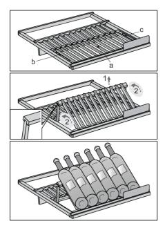
Serving bottle shelf also allows storing bottles in two positions: horizontally or tilted/inclined. The front part of the shelf (a) can be lifted (1) and supported by the rotated (2) lateral supports (b, c). Up to 6 Bordeaux bottles can be placed on the front side of the shelf.
