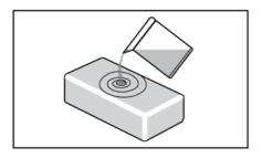
Fill the box with 0.5 litre of tap water and place it in the relevant zone. There are no preferrable positions, as long as it is placed in the correct zone.
