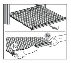
To remove a shelf from the appliance, fully extend the telescopic rails (1), and then vertically lift the shelf (2) to remove it from the rails. When removing the shelf, you can experience some resistance because of the fixation with the pin on the front side. Take care not to damage the door gasket.
