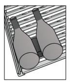
In some cases, during opening/closing of the shelf, bottles are not properly positioned or stopped and they can move. To prevent movement of the bottles on the shelf, it is recommended to use the accessory 'bottle stopper' (a) included in the appliance equipment.
