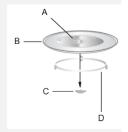
A-glass tray; B-hub (under); C-turntable shaft; D-turntable ring
