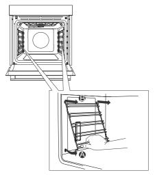
A Hold the guides by the bottom side and pull them towards the center of the oven cavity.
