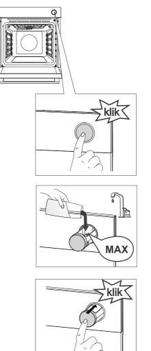
**1** Remove the water tank from the housing by pressing the knob. When you press the knob, the tank jumps out.
