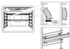
The click-on pull-out guide can be inserted into any space between two wire guides. Place the guide symmetrically onto the wire guides on the left and the right side of the oven cavity. First, hook the upper clip of the guide under the wire of the wire guide. Then, press the lower clip into the right position until you hear a CLICK.
