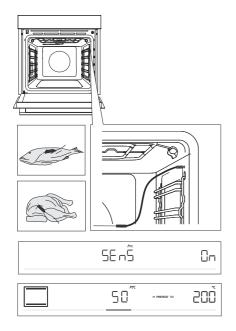
**1** Stick the metal end of the probe into the thickest part of the food.
