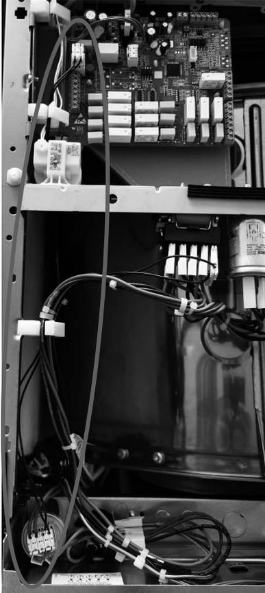
3. Route power supply wiring harness to rear side of washing machine, under electro component bracket and connect it to input filter as shown on picture above.
