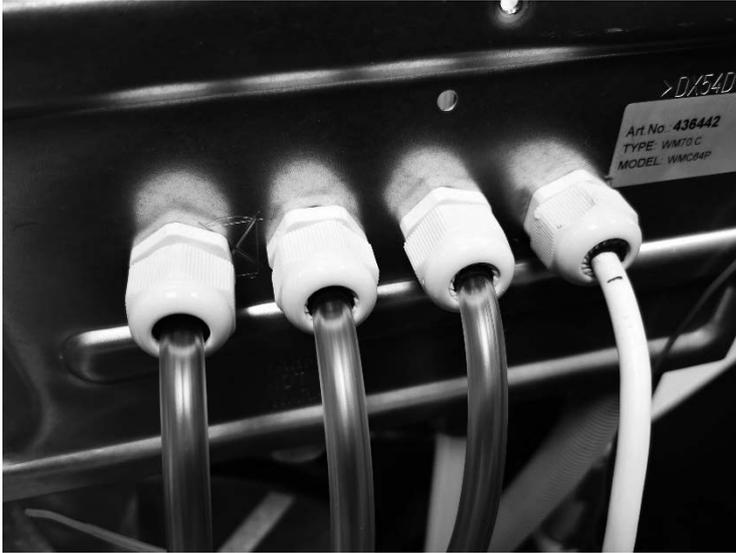
13. Where cable is routed through grommet, screw the grommet nut very tight, the cable pullout force of **>100N** and rotational force of **≥0,35Nm** without movement must be assured! Grommets with hoses must be tightened carefully, make sure that the hoses do not get deformed.
