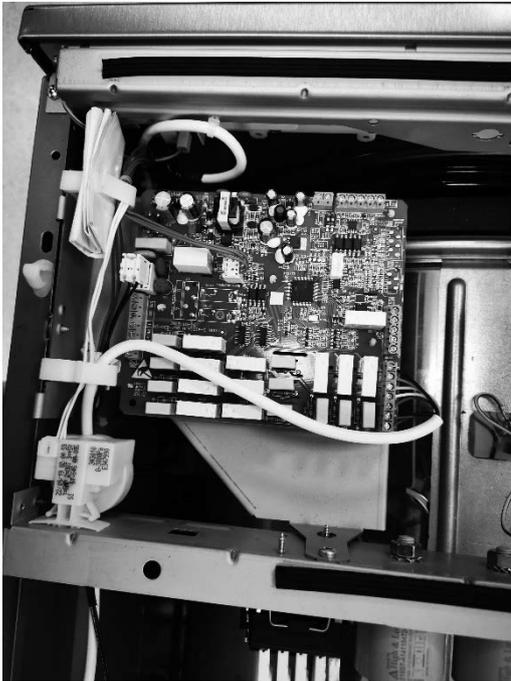
1. Install kit in washing machine on position as shown on picture above, route the harness that is in WM through cable holders (white plastic holders).
