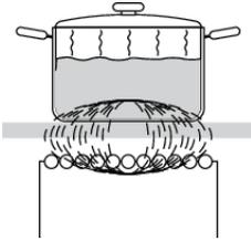
A magnetic field is generated in the appliance. By placing a pan with an iron base on a cooking zone, a current is induced in the pan base. This induced current generates heat in the base of the pan.
