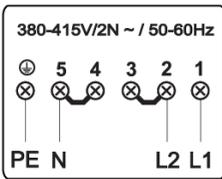
2 phases, 1 neutral conductor (380–415 V 2N~, 50-60 Hz).
