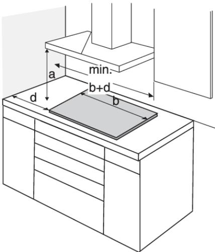
Use of solid wood corner trims on worktops behind the cooking hob is only allowed if the clearance between the trim and the cooking hob is no smaller than indicated on the installation plans.
