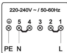
1 phase, 1 neutral conductor (220–240 V~, 50-60 Hz)
