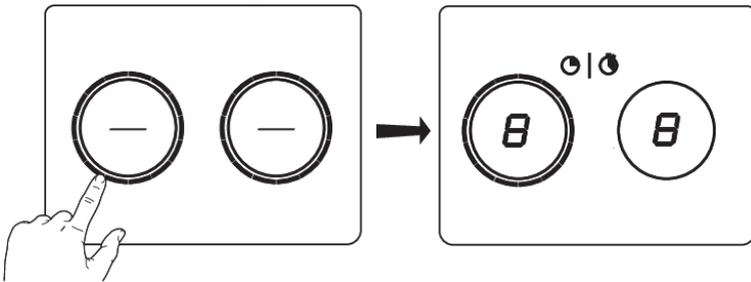
Two adjacent square cooking zones can be merged into a single large cooking zone. Pan position recognition is activated automatically after the appliance is switched on. When a pan will be placed on the hob, the pan recognition function will recognize its position and automatically connect the bridge cooking zones depending on the size of the pan (only when hob was already switched on).
