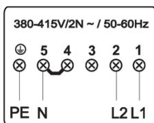
2 phases, 1 neutral conductor (380–415 V 2N~, 50-60 Hz)
