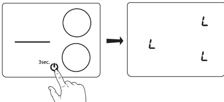
Cooking hob controls can be locked to prevent it from being switched on inadvertently.
