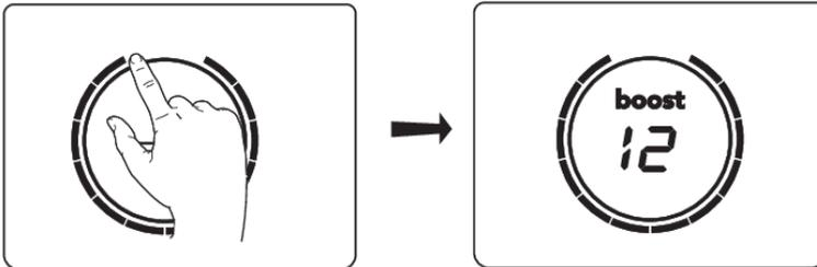
Rapid cooking, boost can be activated for any cooking zone. This will allow you to rapidly heat large amounts of food using extra power. Boost is active for no more than 10 minutes; then, the power level is automatically decreased to 12. If the cooking hob is not too hot, the boost can be reactivated again for 10 minutes after it is switched off.
