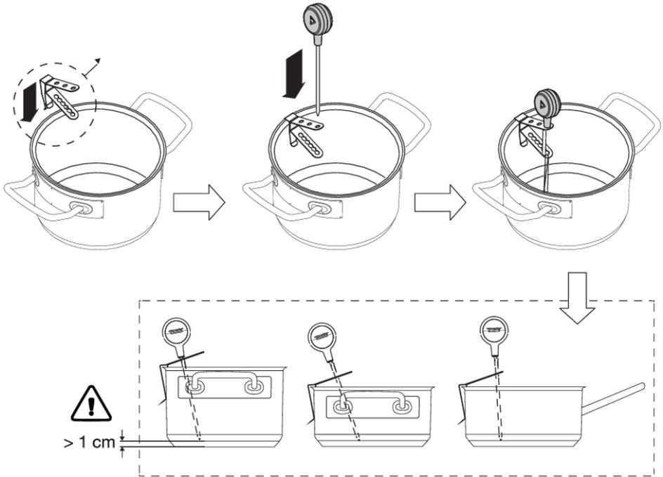
1. Slide the suspension bracket over the pan edge.
