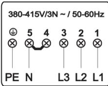
3 phases, 1 neutral conductor (380–415 V 3N~, 50-60 Hz).
