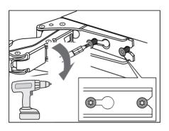
11. Tighten the screws. The screws should be tightened to a torque of 6.2 Nm.
