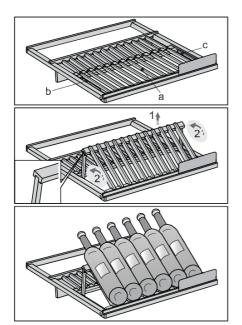
Serving bottle shelf also allows storing bottles in two positions: horizontally or tilted/inclined. The front part of the shelf (a) can be lifted (1) and supported by the rotated (2) lateral supports (b, c). Up to 6 Bordeaux bottles can be placed on the front side of the shelf.
