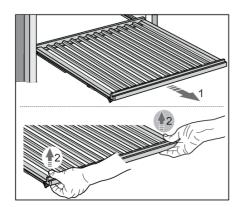
To remove a shelf from the appliance, fully extend the telescopic rails (1), and then vertically lift the shelf (2) to remove it from the rails. When removing the shelf, you can experience some resistance because of the fixation with the pin on the front side. Take care not to damage the door gasket.
