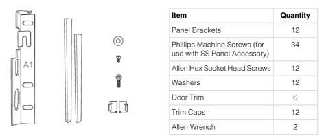
Attach A1 - F1 brackets to the door panels in the locations identified below. Custom panels must have pre-drilled holes as shown in Door Panel Templates. If you purchased an SS Panel Accessory, use the Phillips machine screws to attach the brackets to the SS door panels. For custom panels, use an appropriate wood screw.
