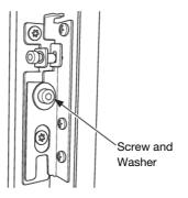
8. Shift the panel side to side to ensure even gaps with the adjacent cabinetry on both sides.
