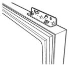
13. With another person holding the door in place, align the holes in the door hinge bracket with the holes in the hinge. Install the screws to the top hinge first.
