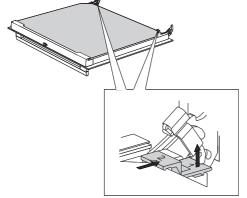
Slightly lift the supports on the left and right side of the door (marking 1 on the support) and pull them away from the glass pane (marking 2 on the support).
