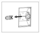
2 Remove the halogen bulb.
