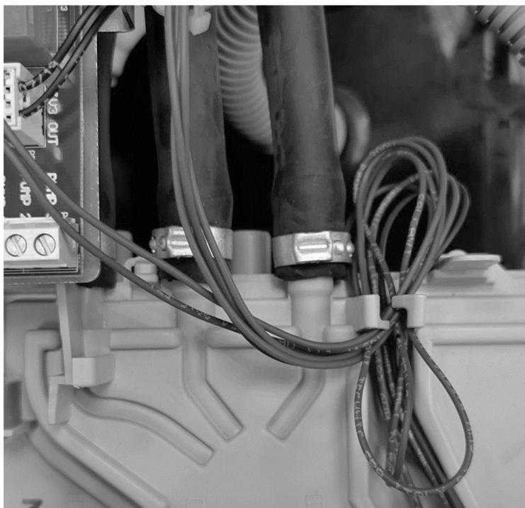
5. On detergent dispenser tuck away the wires that are coming from control unit to relay board that are now too long.
