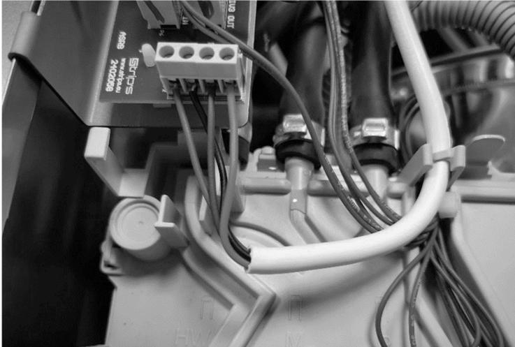
10. Connect the wires (cable) for external dosing pumps to relay board terminal.
