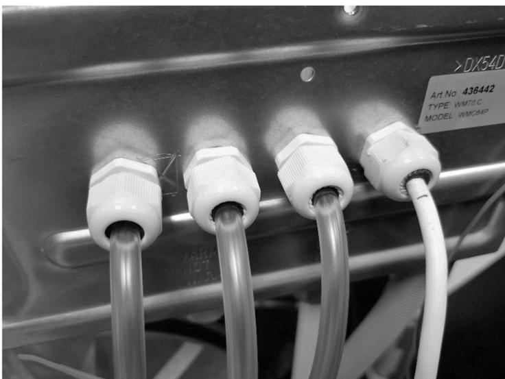
13. Where cable is routed through grommet, screw the grommet nut very tight, the cable pull out force of **>100N** must be assured! Grommets with hoses must be tightened carefully, make sure that the hoses do not get deformed.
