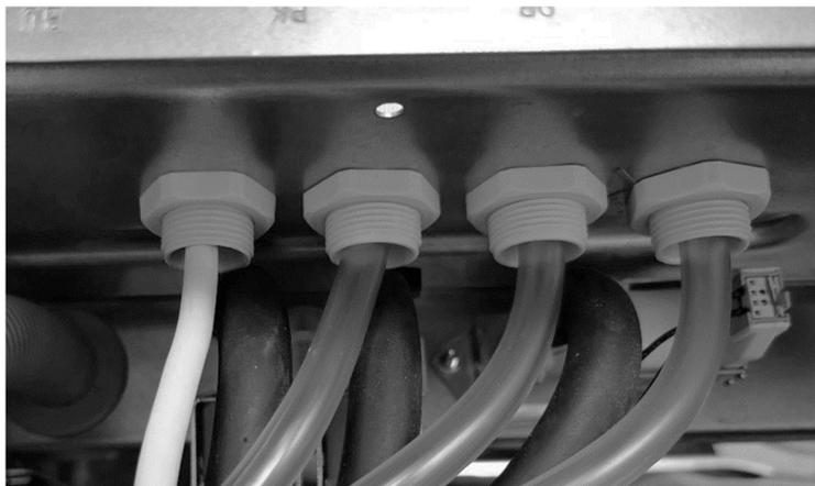
8. Install all the hoses and cable through grommets as shown on picture above.
