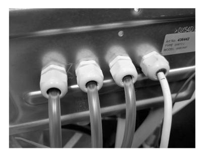
13. Where cable is routed through grommet, screw the grommet nut very tight, the cable pull out force of **>100N** must be assured! Grommets with hoses must be tightened carefully, make sure that the hoses do not get deformed.
