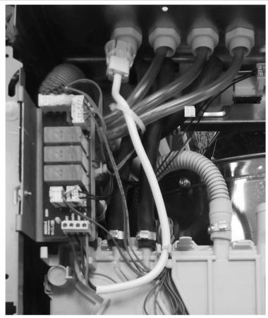
12. Route the cables as shown on picture above, use cable tie to hold the cables and hoses together.
