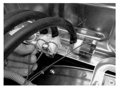
2. Disconnect the cables which come from the control unit to the valves from the inlet valves. Take note which connector is connected to valve 1 (IV1), 2 (IV2) and valve 3 (IV3).
