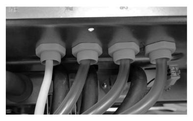
8. Install all the hoses and cable through grommets as shown on picture above.
