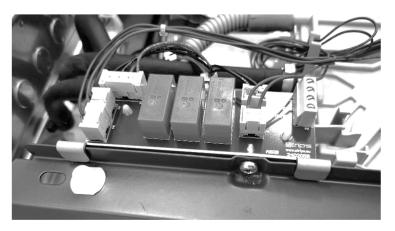
4. Position the card on back left side (next to detergent dispenser) and fasten it with screw.
