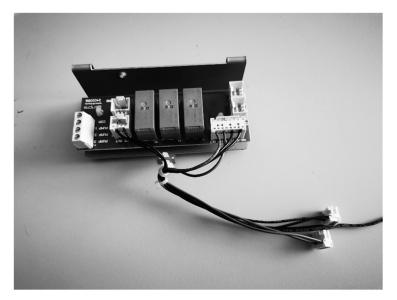
1. Connect the wiring harness to relay board and fixate it with cable tie as shown on the picture above.
