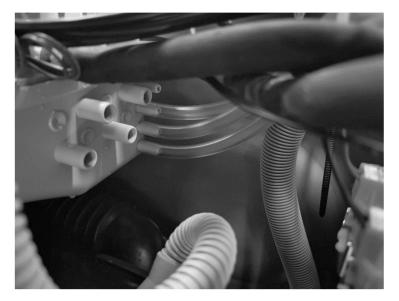
9. You can connect the hoses to small holes (like on the picture) or to larger holes nearby. Drill the holes on detergent dispenser where the hoses will be connected with an appropriate size drill bit and then connect hoses as shown on picture above.
