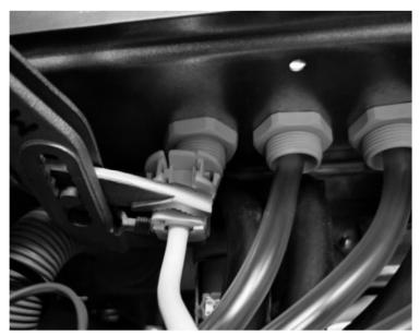
11. Use strain relief that was in the kit, mount it to the cable from inner side of washing machine right next to grommet, make sure no gap is left between grommet and strain relief. Squeeze strain relief tight with appropriate tool (pliers).
