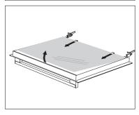
$\bf 3$  Slightly lift the door glass and remove it from the clips on the bottom side of the door.
