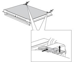
I Slightly lift the supports on the left and right side of the door (marking 1 on the support) and pull them away from the glass pane (marking 2 on the support).
