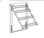
Mount the guides onto the catalytic insert.
