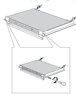
1 Undo the holder screws on both sides of the door.
