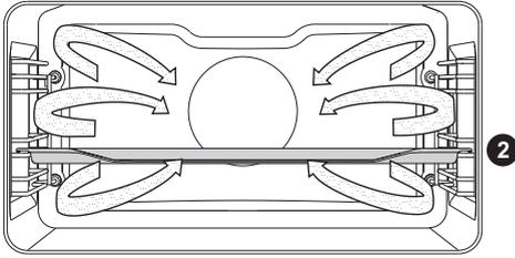
Water from the steam generator enters the oven cavity in the form of steam.
