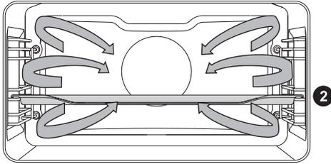
Round heater and the fan will operate. The fan installed on the back wall of the oven cavity makes sure the hot air constantly circulates around the meat, vegetables, or pastry.
