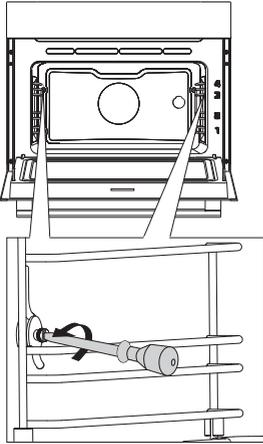
**1** Undo the screw. Use a screwdriver.
