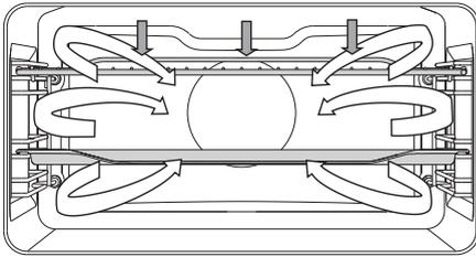
In this operating mode, the grill heater and the fan operate simultaneously. Suitable for grilling meat, fish, and vegetables.
