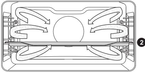
Water from the steam generator enters the oven cavity in the form of steam. In addition, round heater with fan operates to provide continuous circulation of the hot air and steam.
