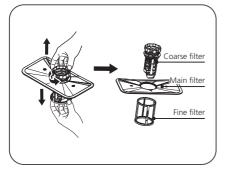
The filter system consists of a coarse filter, a flat (Main filter) And a microfilter (Fine filter).
