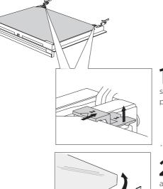
Slightly lift the supports on the left and right side of the door (marking 1 on the support) and pull them away from the glass pane (marking 2 on the support).
