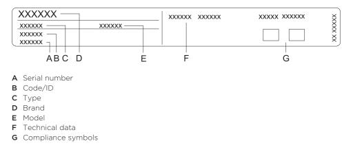
The rating plate indicating the basic information about the appliance is located at the edge of the oven and it is visible when the oven door is opened.
