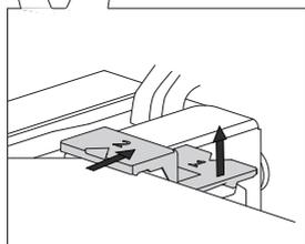
**1** Slightly lift the supports on the left and right side of the door (marking 1 on the support) and pull them away from the glass pane (marking 2 on the support).
