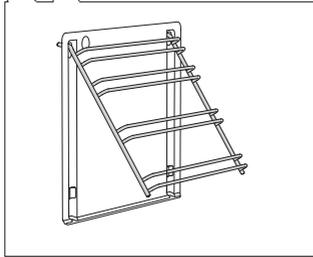
**1** Mount the guides onto the catalytic insert.
