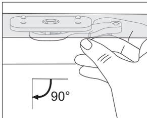
**3** To reactivate the door lock, open the oven door and use your right-hand index finger to pull the lever towards you.
