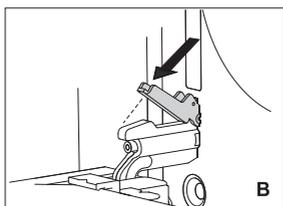
**B** If the appliance is fitted with the GentleClose system, flip the door latch back to a 90° angle (Figure 2).
