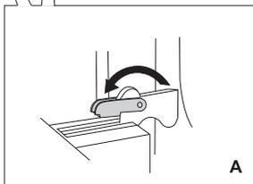
**2** **A** Rotate the stoppers all the way back (in case of conventional closing).
