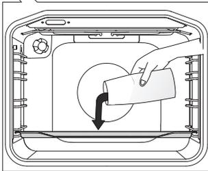
**2** Pour 0.6 l of water into a glass or shallow baking dish and insert it into the lower guide.
