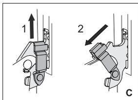
**C** If the appliance is fitted with the GentleClose system, slightly lift the door latches and pull them towards you.
