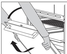
**3** Slowly close the door until the latches are aligned with the slots. Slightly lift the door and pull it out from both hinge slots on the appliance.
