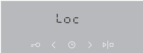
**3** After a certain period of time, oven door will be automatically locked for your safety. "Loc" will appear on the display unit (for 3 seconds).
