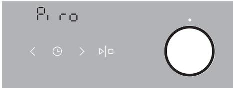
**2** Rotate the TEMPERATURE ADJUSTMENT KNOB all the way to the right to the "P" sign. "Pyro" will flash on the display unit, along with the indication of pyrolytic cleaning duration.
