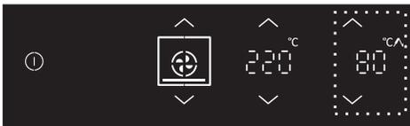
When the probe is connected, "Prob" will appear on the display unit. Set the desired temperature. Touch the START key.
