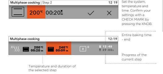
By touching the START key, the oven first starts operating according to step 1. (The progress bar on the bottom of the display indicates the current step of the baking process). When a certain time expires, step 2 is activated and then step 3 if it was selected.
