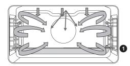
This system uses a combination of microwaves and grill with fan to cut the cooking time.
