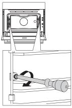
**1** Undo the screw. Use a screwdriver.
