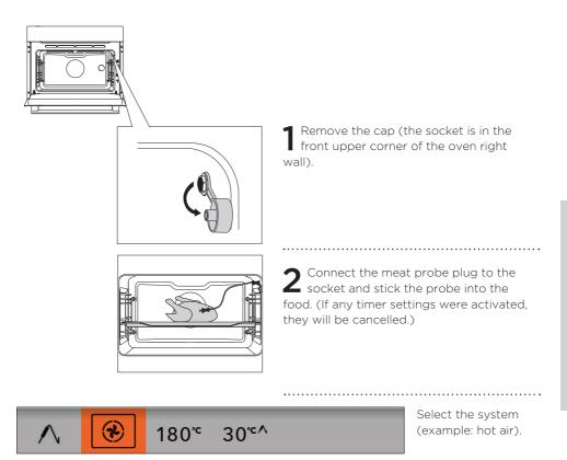
Preset temperature and probe temperature will be displayed. Set the cooking system and temperature, and the final temperature of the dish. Touch the START key.
