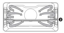
Round heater and the fan will operate. The fan installed on the back wall of the oven cavity makes sure the hot air constantly circulates around the meat, vegetables, or pastry.
