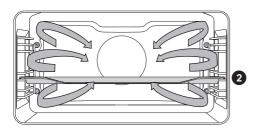
Round heater and the fan will operate. The fan installed in the back wall of the oven cavity makes sure the hot air constantly circulates around the roast or pastry.
