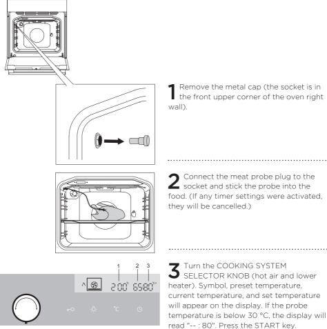
Remove the metal cap (the socket is in the front upper corner of the oven right wall).
