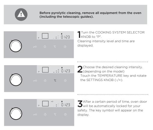
During cleaning, the appliance becomes very hot on the outside. Never hang flammable objects like kitchen cloths or similar on the front panel of the appliance.
