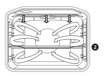
In this operating mode, the grill heater and the fan operate simultaneously. Suitable for grilling meat, fish, and vegetables.
