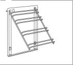
Mount the guides onto the catalytic insert.
