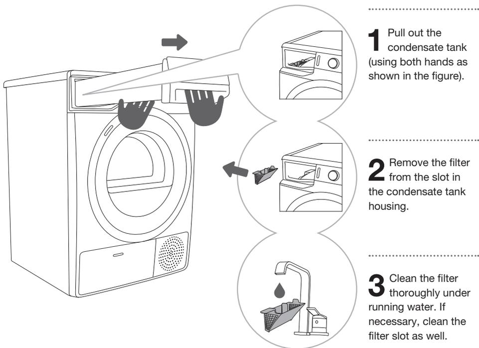
⚠️ Replace the filter correctly into the slot (otherwise, the filter will not perform its function, which may result in clogging of the system).
