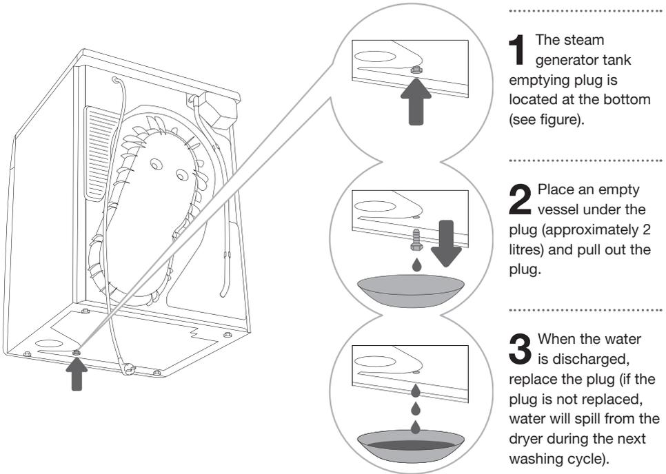
⚠ Emptying the steam generator tank is a task that should be conducted by at least 2 persons.
