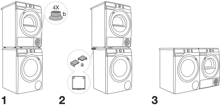
⚠ At least two persons are required to install the tumble dryer on top of a washing machine.
