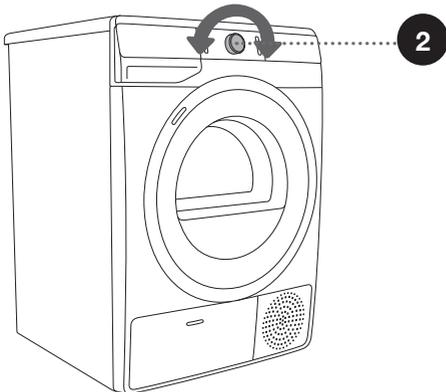
⚠ The programme selector knob (2) will not rotate automatically during operation.
