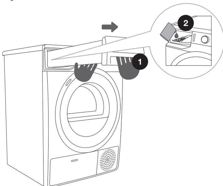
**1** Pull out the condensate tank (using both hands as shown in the figure).
