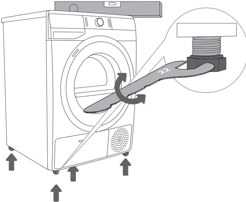
⚠ Floor on which the dryer is placed must have a concrete base. It should be clean and dry; otherwise, the dryer may slide. Also clean the adjustable feet.
