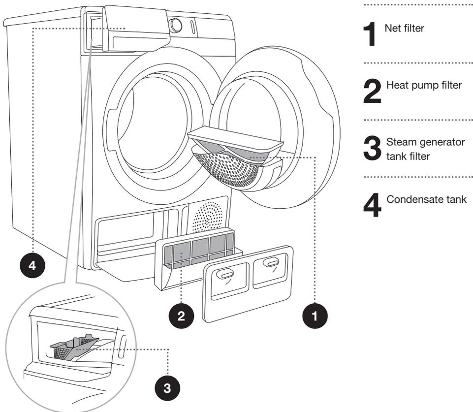
**⚠** The dryer may never be operated without the filters in place or with damaged filters, as excessive amount of accumulated fibres from the fabric could cause malfunction or failure of the dryer.
