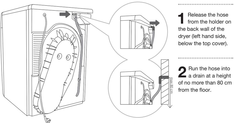
**1** Release the hose from the holder on the back wall of the dryer (left hand side, below the top cover).
