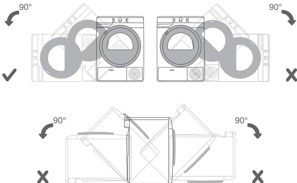
⚠ After installation, wait for 24 hours without moving the appliance before using it for the first time. If the dryer has to be laid down on one of the sides during transport or servicing, place it with its left side, viewing from the appliance front, downwards.
