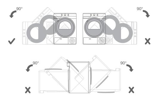
$\dot{\nabla}$  After installation, wait for 24 hours without moving the appliance before using it for the first time. If the dryer has to be laid down on one of the sides during transport or servicing, place it with its left side, viewing from the appliance front, downwards.
