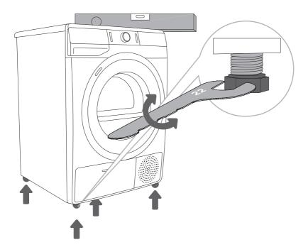
$\dot{\sigma}$  Floor on which the dryer is placed must have a concrete base. It should be clean and dry; otherwise, the dryer may slide. Also clean the adjustable feet.
