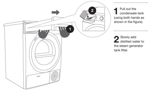
If the steam generator tank is empty, the sign appears and the **STEAM REFRESH** (REFRESH WITH STEAM) programme cannot be run. Later on, as you use your dryer, the system will be filled automatically with condensed water extracted during the drying process.
