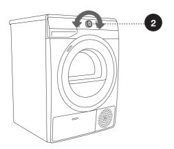
$\dot{\nabla}$  The programme selector knob (2) will not rotate automatically during operation.
