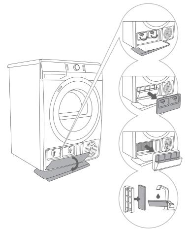
• Open the outer cover. Hold the levers on the inside cover and rotate them upwards. Remove the inside cover.
