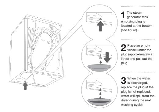
'ġ' Emptying the steam generator tank is a task that should be conducted by at least 2 persons.
