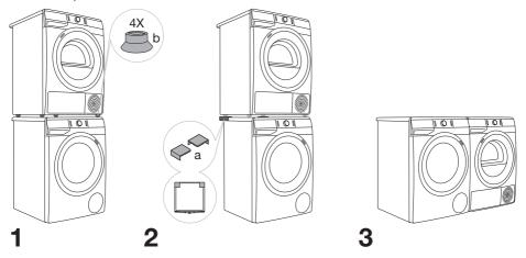
ở At least two persons are required to install the tumble dryer on top of a washing machine.
