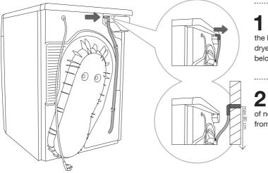
Release the hose from the holder on the back wall of the dryer (left hand side, below the top cover).
