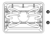
In this operating mode, the grill heater and the fan operate simultaneously. Suitable for grilling meat, fish, and vegetables.
