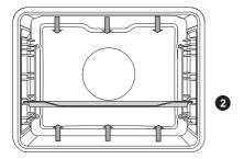
The heaters in the bottom and in the ceiling of the oven cavity will radiate heat evenly into the oven interior.
