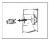
2 Remove the halogen bulb.
