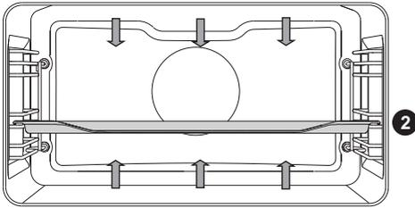
The heaters in the bottom and in the ceiling of the oven cavity will radiate heat evenly into the oven interior.
