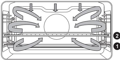
In the Auto Roast mode, the upper heater will operate in combination with the grill heater and the round heater. It is used for roasting all types of meat.
