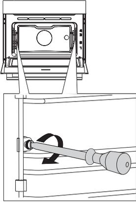
**1** Undo the screw. Use a screwdriver.
