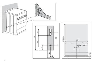
Dimensions in the parenthesis represent built-in measures of the support bracket without the additional support. If the supplied element protecting the appliance from tipping over cannot be firmly secured to your wall with the screws and the wall plugs supplied, use other fittings to secure the bracket in such way that it cannot be pulled out from the wall.
