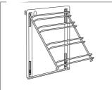
Mount the guides onto the catalytic insert.
