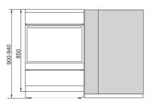
The walls or furniture adjacent to the appliance (floor, rear kitchen wall, side walls) have to be temperature-resistant to at least 90  $^{\circ}$ C.
