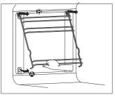
**A** Hold the guides by the bottom side and pull them towards the center of the oven cavity.
