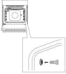
1 Undo the metal cap from the socket in the upper corner of the left oven cavity wall.
