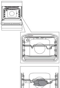
Insert the skewer support into the 3rd guide from the bottom and place the deep tray into the bottom (1st) guide to serve as a drip tray.
