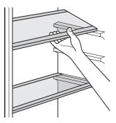
The walls of the refrigerator are equipped with a series of runners so that the shelves can be positioned as desired.
