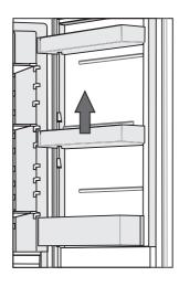
To permit storage of food packages of various sizes, the door balconies can be placed at different heights. To make these adjustments proceed as follows: gradually pull the balcony in the direction of the arrows until it comes free, then reposition as required.
