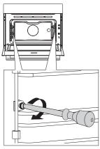
**1** Undo the screw. Use a screwdriver.
