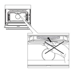
Never use aggressive cleaners, abrasive cleaners, abrasive sponges, stain and rust removers etc. on the oven ceiling cover.
