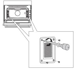
1 Undo the four screws on the cover. Remove the cover and the glass.
