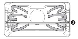
Round heater and the fan will operate. The fan installed in the back wall of the oven cavity makes sure the hot air constantly circulates around the roast or pastry.
