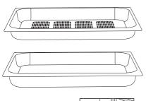
**STEAM SET (INOX)** is used for steam cooking. Place the perforated tray in the middle level and the drip tray one level below.
