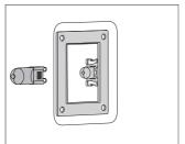
**?** Remove the halogen bulb.
