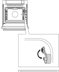
Remove the cap (the socket is in the front upper corner of the oven right wall).
