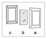
There is a gasket on the cover which should not be removed. Do not allow the gasket to be detached from the cover. The gasket should fit correctly onto the oven cavity wall.
