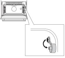
Remove the cap (the socket is in the front upper corner of the oven right wall).
