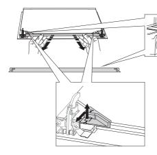
Slightly lift the supports on the left and right side of the door (marking 1 on the support) and pull them away from the glass pane (marking 2 on the support).
