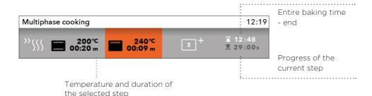
By touching the START key, the oven first starts operating according to step 1. (The progress bar on the bottom of the display indicates the current step of the baking process). When a certain time expires, step 2 is activated and then step 3 if it was selected.
