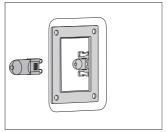
**?** Remove the halogen bulb.
