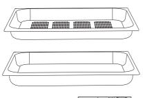
**STEAM SET (INOX)** is used for steam cooking. Place the perforated tray in the middle level and the drip tray one level below.
