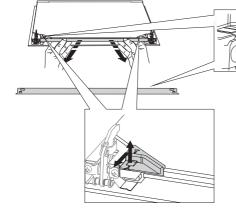
1 Slightly lift the supports on the left and right side of the door (marking 1 on the support) and pull them away from the glass pane (marking 2 on the support).
