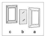
There is a gasket on the cover which should not be removed. Do not allow the gasket to be detached from the cover. The gasket should fit correctly onto the oven cavity wall.
