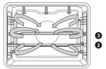
In the Auto Roast mode, the upper heater will operate in combination with the grill heater and the round heater. It is used for roasting all types of meat.
