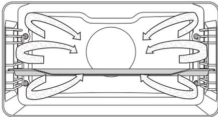
Water from the steam generator enters the oven cavity in the form of steam. In addition, round heater with fan operates to provide continuous circulation of the hot air and steam.
