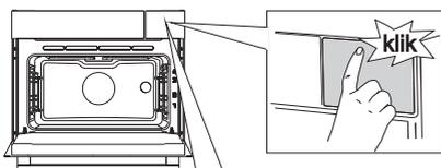
**1** Press on the spot with the sticker to open the tank door.
