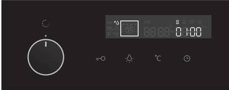
Turn the COOKING SYSTEM SELECTOR KNOB to defrosting. TIME will be displayed. This time setting can be adjusted. Press the START key.
