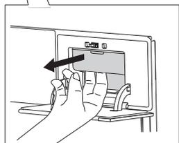
**2** Remove the water tank from the housing by grabbing the notch.
