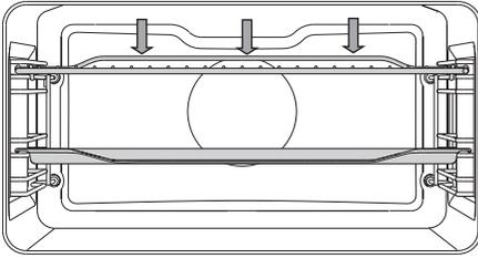
When grilling food, the upper heater and the grill heater fitted on the ceiling of the oven cavity will operate.
