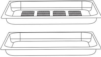
**STEAM SET (INOX)** is used for steam cooking. Place the perforated tray in the middle level and the drip tray one level below.
