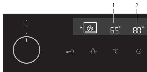
**3** Turn the COOKING SYSTEM SELECTOR KNOB (hot air and lower heater). The symbol, oven cavity set temperature and meat probe set temperature will appear on the display unit. Press the START key.
