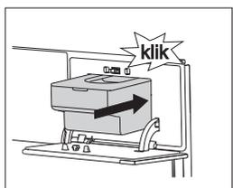
**4** Push the water tank back into the housing to the final position (until the short click). Then, press the tank door to close it.
