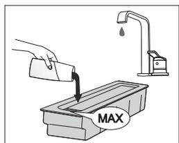
**3** Open the lid. Wash the tank with water. Re-assemble the tank. Before use, add fresh water up to the MAX marking on the tank.
