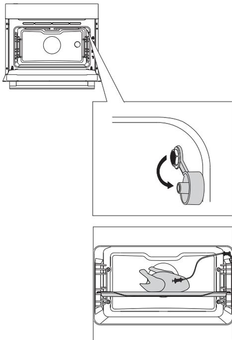
**1** Remove the metal cap (the socket is in the front upper corner of the oven right wall).
