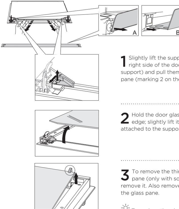
**1** Slightly lift the supports on the left and right side of the door (marking 1 on the support) and pull them away from the glass pane (marking 2 on the support).
