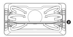
Water from the steam generator enters the oven cavity in the form of steam.
