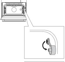
Remove the cap (the socket is in the front upper corner of the oven right wall).
