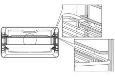
In case of wire guides, the tray should always be inserted into the groove between the two wire profiles.
