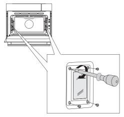
Use a flat screwdriver to release the bulb cover and remove it.
