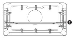
The heaters in the bottom and in the ceiling of the oven cavity will radiate heat evenly into the oven interior.
