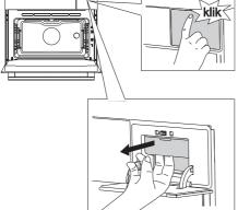
Press on the spot with the sticker to open the tank door.
