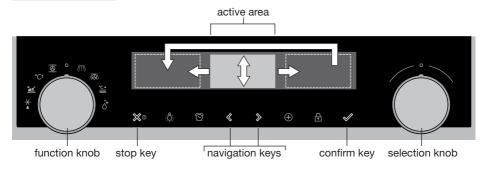
By turning the function knob away from the 0-position, the icon of the chosen main function is lit. The display will show the icon and name of the activated function for about 1,5 seconds. Next you will see the chosen main function and sub-function at the top of the display in the feedback bar. Also the function settings mode will become active (grey background). In this activated area you can select your settings using the selection knob.
