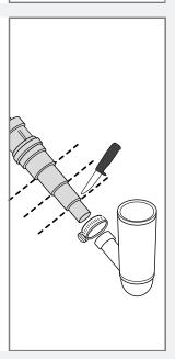
The drain hose can also be connected to a connection nipple on the sink's water trap. The connection nipple must have an internal diameter of at least 1/2". The water trap must be ventilated.
