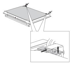
I Slightly lift the supports on the left and right side of the door (marking 1 on the support) and pull them away from the glass pane (marking 2 on the support).
