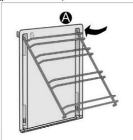
Mount catalytic inserts onto the wire guides. The upper part of the guides must be mounted into the upper openings "A" in the catalytic inserts.
