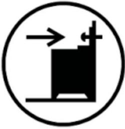
**WARNING:** In order to prevent tipping of the appliance, stabilising means must be installed. Refer to the instructions for installation.
