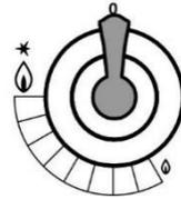
Cooking power levels are indicated on the knobs with a large and a small flame symbol. Rotate the knob over the large flame position (🔥) to the small flame position (🔥) and back. Operating range is between the two flame symbols.
