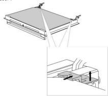
Slightly lift the supports on the left and right side of the door (marking 1 on the support) and pull them away from the glass pane (marking 2 on the support).
