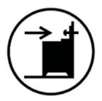
WARNING: In order to prevent tipping of the appliance, stabilising means must be installed. Refer to the instructions for installation.
