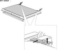
Slightly lift the supports on the left and right side of the door (marking 1 on the support) and pull them away from the glass pane (marking 2 on the support).
