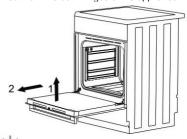
Provide these steps in reverse order at returning the door back. If the door does not open or close properly, make sure, that the hinges are correctly located on their hooks.
