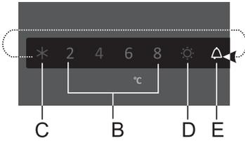
If the temperature inside the appliance is too high, acoustic alarm will be activated (**intermittent tone**) and the **E** symbol will flash.
