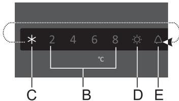
To activate the intensive freezing (freezer boost) function, press the **A** key several times until the symbol **C** lights up.
