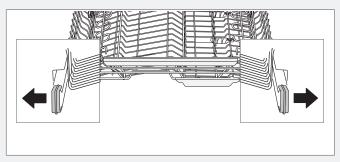
Pull out the top cutlery tray. Push the top spray arm up and turn the spray arm bearings counterclockwise to remove the spray arm.
