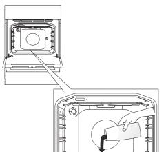
Ignite the gas in the oven and rotate the system selector knob to the AQUA CLEAN position ow
