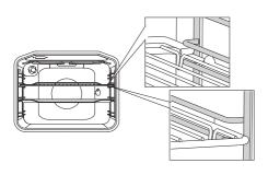
The grid or the tray should always be inserted into the groove between the two wire profiles.
