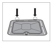
Insert it into the holes left and right at the back and fixed at the front to prevent it from moving when the oven is used the next time.
