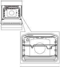
Insert the skewer support into the 3rd guide from the bottom and place the deep tray into the bottom (1st) guide to serve as a drip tray.
