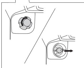
Release the bulb cover and remove the bulb.
