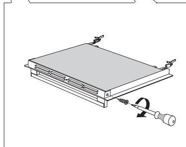
**1** Undo the holder screws on both sides of the door.
