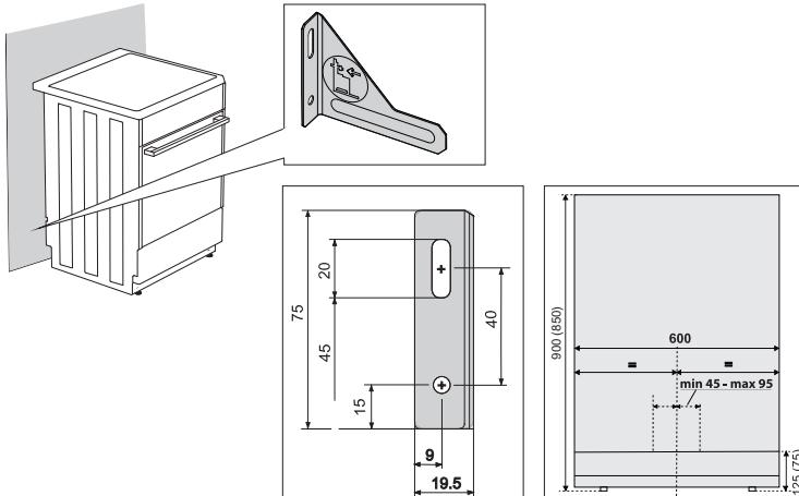
Dimensions in the parenthesis represent built-in measures of the support bracket without the additional support. If the supplied element protecting the appliance from tipping over cannot be firmly secured to your wall with the screws and the wall plugs supplied, use other fittings to secure the bracket in such way that it cannot be pulled out from the wall.
