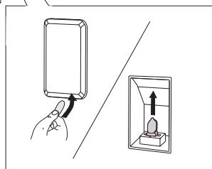
Use a flat screwdriver to release the bulb cover and remove it. Remove the bulb.
