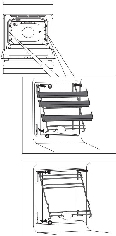
**A** Hold the guides at the bottom side and pull them towards the center of the oven cavity.
