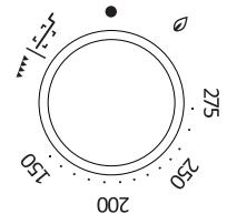
Rotate the knob (left and right) to select the cooking system (see program table).
